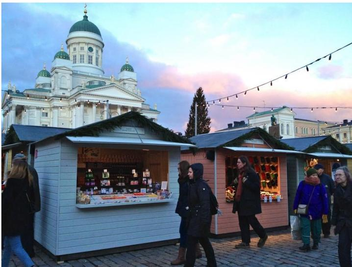
Basic cabin dimensions: width approx. 2.5 m, depth approx. 2.0 m. Each cabin is equipped with a sales desk, awning and three shelves along the back wall. The door is on the side of the cabin and can be locked using your own padlock.
